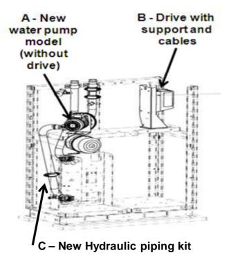
**<u>Caution</u>** : Location and installation of the external drive must be done in the most appropriate place into the unit.
